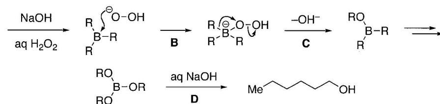
**A:** Hydroboration through a four-membered transition state. **B:** Attack of a hydroperoxide anion to the borane to form an ate complex. **C:** Migration of an alkyl group. **D:** Hydrolysis of the borate.
